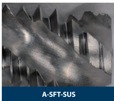
■1,000穴加工後 Cutting edge after tapping 1,000 holes
